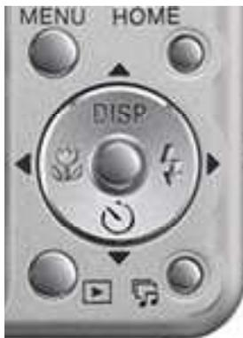
**The bottom half:** There is a circular disc with four buttons around it and one in the middle. While it's not immediately clear what the difference between "Menu" and "Home" is (-), after one try, with the on-screen messages, it's easy to remember that "Menu" is for adjusting picture settings and "Home" brings up options relating to the camera itself. (~)
