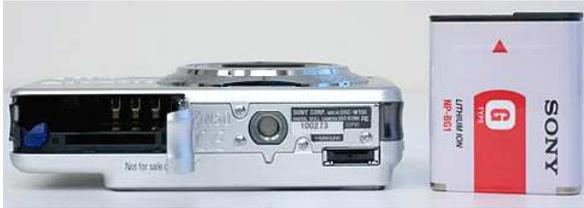
The door to where the battery and memory card are inserted has raised bumps in the shape of an arrow head making it obvious how to open it (+). And the shape of the battery and the opening constrain the battery's insertion. (+)
